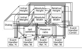
**Figure 3.** The incidental data structure formed as the dependencies between the UI components and event handlers in an objectoriented implementation of the user interface logic of dialog shown in Figure 2. The edges correspond to the relations "event handler writes to a value" or "event handler reads a value."
