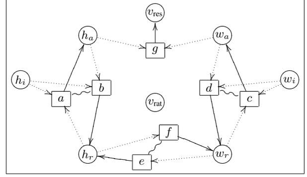
**Figure 6.** A constraint system for command parameter synthesis for an image-resize command. The rectangles represent method vertices. Dotted arrows are inputs to methods, solid arrows outputs from methods.
